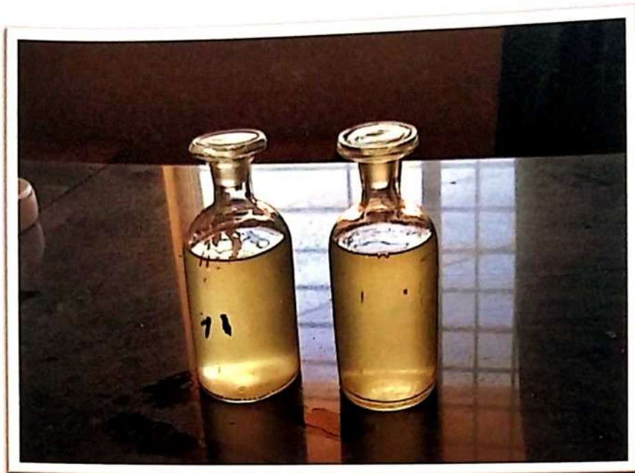
Before addition of \text{MnSO}_4 and alkaline KI in water sample for estimation of DO
