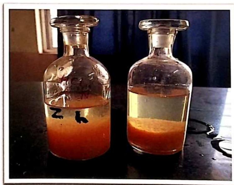
After addition of \text{MnSO}_4 and alkaline KI in water sample for estimation of DO
