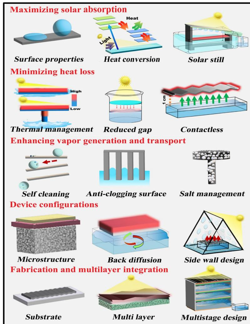
**Figure 3.** Illustrations of device assembly strategies to achieve clean water production from sea water.
