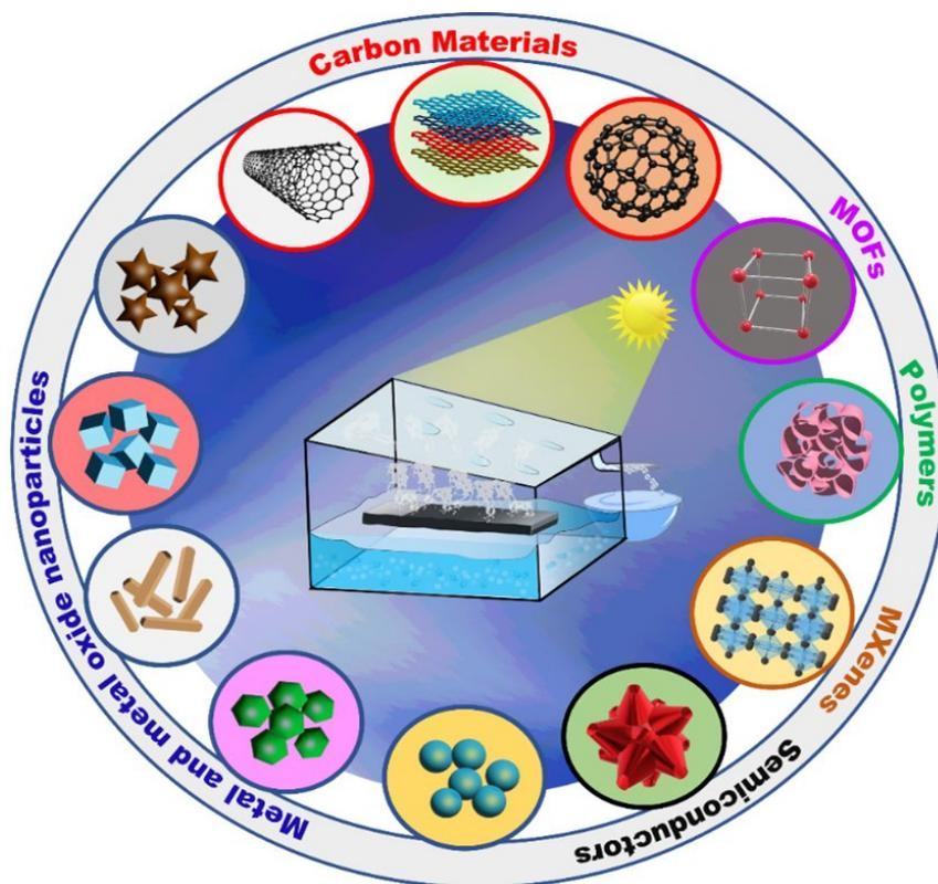
Figure 1. Various types of photothermal materials used in SIE.
