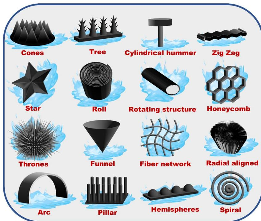
Figure 4. Illustration of various solar water evaporators with different surface structures.
