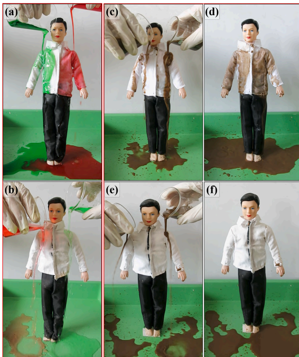
Fig. 8. The colored water dropped on (a) uncoated and (b) coated cotton fabric. Muddy water dropped on (c-d) uncoated and (e-f) coated cotton fabric..
