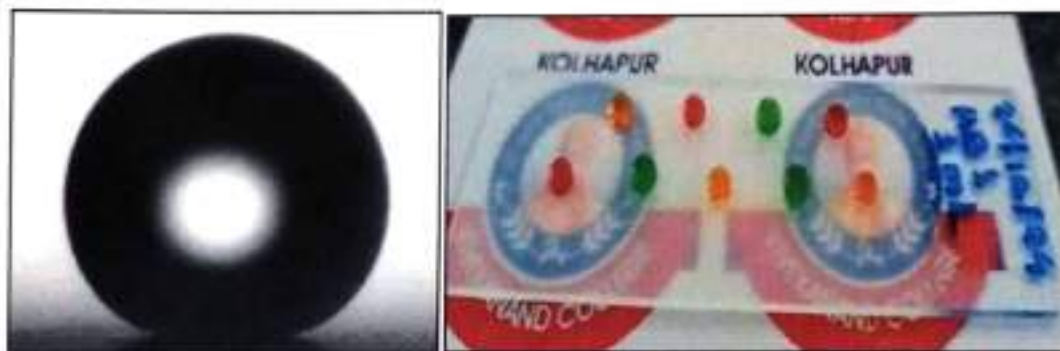
Figure 4.1. Water contact angle image of MP2 sample Figure 4.2. Optical image of colored water droplets on MP2 sample
