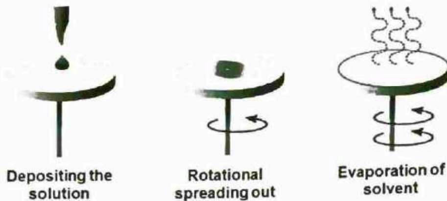
Figure 2 : Spin coating process
