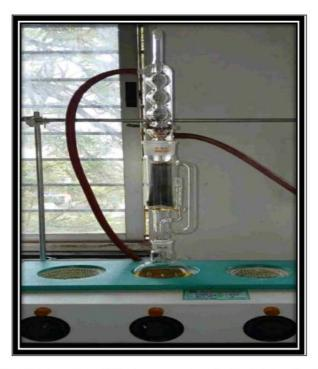
Fig.4 Extraction of Punica granatum by Soxhlet method.
