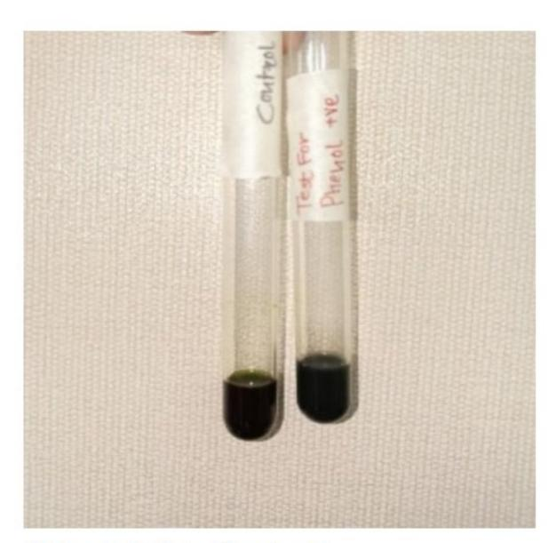
Photograph 13 test for phenol
