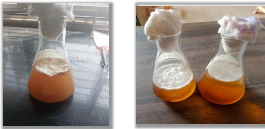
Fig No 9: Formation of thick, firm cellulose layer during prolonged fermentation stage
