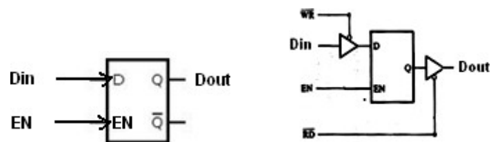
(a) D latch (b) Latch with tri-state buffers
